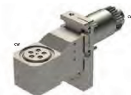
STAR2-GSW-210 Modular Thread Whirling Ring: Utilis Output: 1:1 7 or 9 Insert Cutter, Flight Circle Ø6mm Adjustable ±10°
