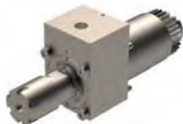
STA-SR20J-GSC-010-HP Cross Drill/Mill Collet Size: ER16 Output: 1:1 Coolant-Thru 2175psi Max
