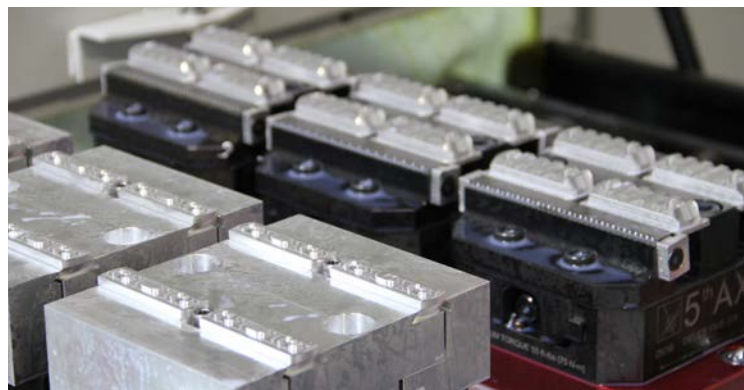
Machinable jaws available for second operations.
